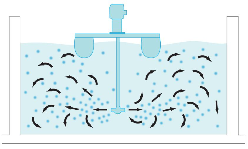
Flow throughout entire tank volume ensures optimum mixing and gas transfer
